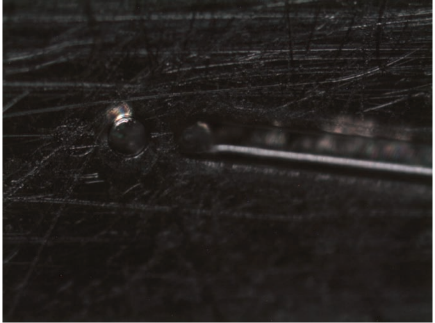
Figure 5. Microscopic holes shot out by the laser ablation inductively coupled plasma mass spectrometry. Rose-tinted film fragment owned by DIASTOR team member David Pfluger, measurement by Beat Aeschlimann, ETH Zurich, Laboratory of Inorganic Chemistry, Günther group.
