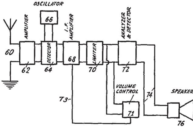
Fig. 14. Block diagram of Clarence Hansell's FM Receiver, 1928. Block diagram shows a limiter circuit, something Armstrong improved upon in his wideband FM system of 1933. Clarence W. Hansell, "Signaling," U.S. Patent No. 1,803,504, application date: 5 October 1928, issue date: 5 May 1931, assigned to RCA.
