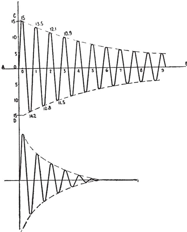
Fig. 7. Damped Waves. Two trains of waves illustrate “feebly damped” (*top*) and “strongly damped” (*bottom*) waves. Dotted lines trace the “envelope” of the wave train peaks. Elmer E. Bucher, *Practical Wireless Telegraphy: A Complete Text Book for Students of Radio Communications* (New York: Wireless Press, 1921), 1.
