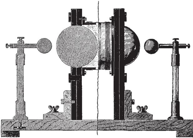
MARCONI'S SPARK-GENERATOR. CROSS SECTION, SIDE VIEW
