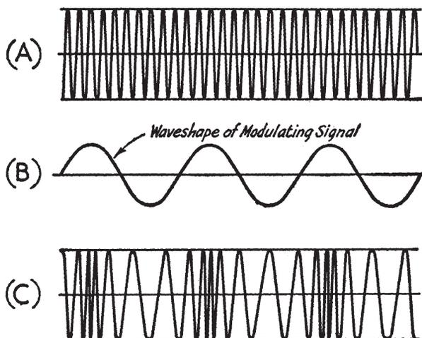
Fig. 3. Frequency-Modulation Waves. FM radio waves on horizontal time scale; (A) an unmodulated carrier; (B) the modulating wave, usually an audio program; and (C) a radiofrequency wave whose wavelength varies with the instantaneous amplitude of B—that is, as B rises and falls in amplitude, the frequency of A rises and falls correspondingly. Adapted from Headquarters Staff of the American Radio Relay League, *The Radio Amateur's Handbook* (Hartford: American Radio Relay League, 1962), 284
