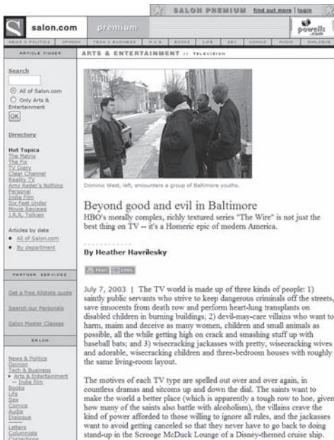
Figure 5: A widely used Web page design. The page banner, navigation header and footer (not shown), and side menu frame the main content of the page.
