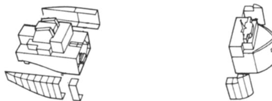
**Because the bow and stern sections of the *Cort* were built at a shipyard on the Gulf of Mexico and had to be brought into the lakes by way of the St. Lawrence River, the sections were limited to a maximum beam of seventy-five feet. Sponsons were later added to the bow and stern to fair them out to the 105-foot width of the vessel's midbody. (Author's collection)**
