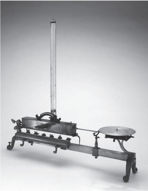
Fig. 2: Pyrometer, an instrument invented by Van Musschenbroek to measure the rate of expansion of metal rods with the temperature. (Museum Boerhaave, Leiden, V09550)
