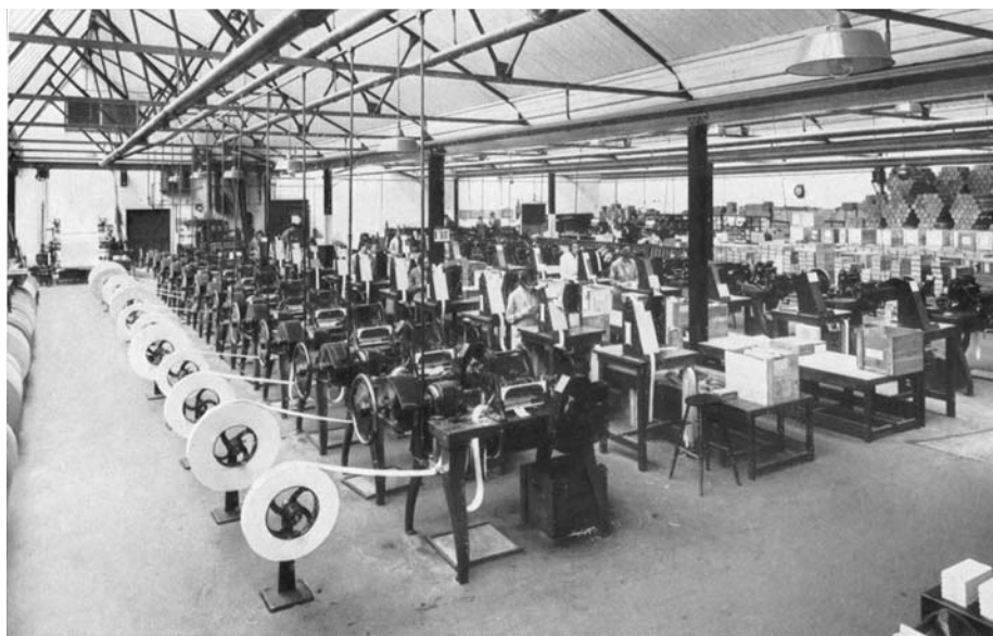
Punched-card production at the Powers-Samas Company in London, 1937. Production of the cards themselves contributed up to a third of the punched-card producers' revenues. ( Powers-Samas Magazine October 1937, 7)
