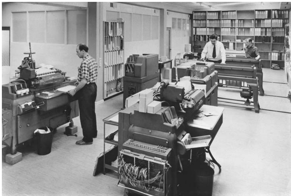
The IBM tabulator Type 405 in the punched-card installation of the Association of Danish Dairies (Mejerikontoret) in 1959. It is the machine to the left operated by the gentleman with the checked shirt and the machine in the center. It remained a core workhorse in IBM punched-card installations until the machines were replaced by computers in the 1960s. (Landbrugets EDB-Center, Risskov, Denmark)
