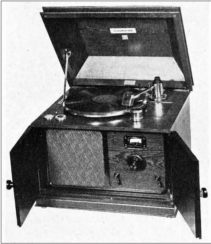
FIG. 1 "A playback machine with an electrical (sound amplification) box, connected with radio reception." (Source: Doegen, Jahrbuch des Lautwesens 1931, 122.)
