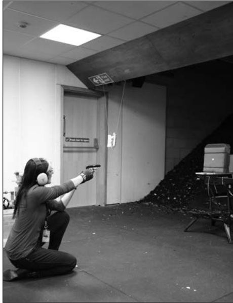
FIG. 14 An original FN Model 1910 pistol (.380 ACP) is fired at a replicated fabric body armour produced to a Casimir Zeglen patent of the late nineteenth century. As well as being able to fire certain collection objects, the Royal Armouries has use of an instrumented test range for the purposes of research and demonstration. (Source: Courtesy of the Royal Armouries Museum, Leeds.)
