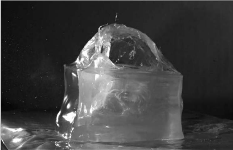
FIG. 13 A block of ballistic gelatin tissue is struck by a load of buckshot from a World War I-vintage Remington Model 1897 "trench gun." This still from some high-speed camera footage shows the maximum extent of the extreme "cavitation" caused by nine .32 caliber lead balls striking close together. (Source: Courtesy of the Royal Armouries Museum, Leeds, UK.)
