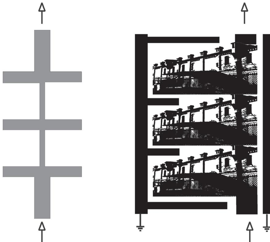
I fabricate the physical circuits by etching thin films of gold on glass plates, typically no more than a few centimeters in size. I use a photographic process to transfer the images into the circuits from digital film output or directly from negatives. These methods are widely used in the electronics industry.
