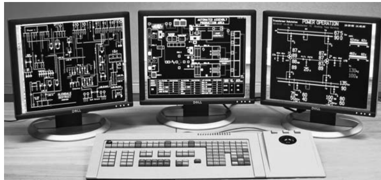
Figure 4. Representative Tessellator images emulated by TessEm software on a modern PC. Note the different symbol sizes. The images are displayed on flat screens in this photo because the product is available now only by emulation. (Courtesy of Newcon Data AB.)
